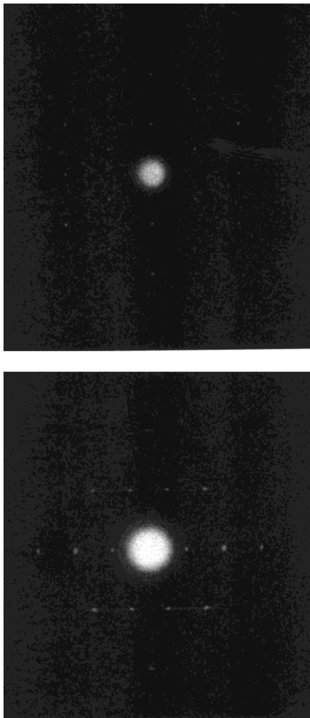
Figure 16. [001] zone electron diffraction patterns of sPS crystallized at T_c = 245\text{ }^{\circ}\text{C} for (a) t_c = 3\text{ min} and (b) t_c = 15\text{ min} from the melt ( T_{\text{max}} = 300\text{ }^{\circ}\text{C} ).
